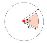
Fig. 2. The sensing model of a camera sensor.
