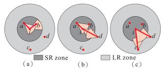
Fig. 6. Three different types of barrier lines. (a)Type SS. (b)Type SL. (c)Type LL.
